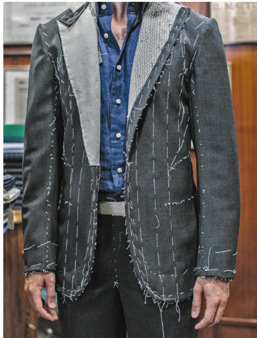
A 'basted fitting' is when you try on a custom suit jacket that has been temporarily stitched together with white basting thread. Initial measurements that were carefully taken during your first fitting were used to create this 'working' jacket. This jacket is used to finetune the fitting. The basted fitting is also the customers first opportunity to try on the custom made suit. It may not look like much, but it will still feel like it was made for you.
